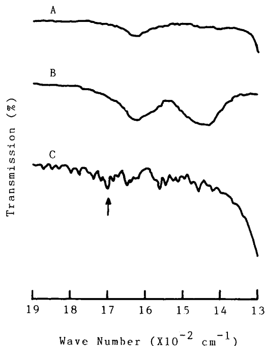
Figure 1 Infrared spectra of (A) PTFE, (B) CPTFE, and (C) WPTFE.
